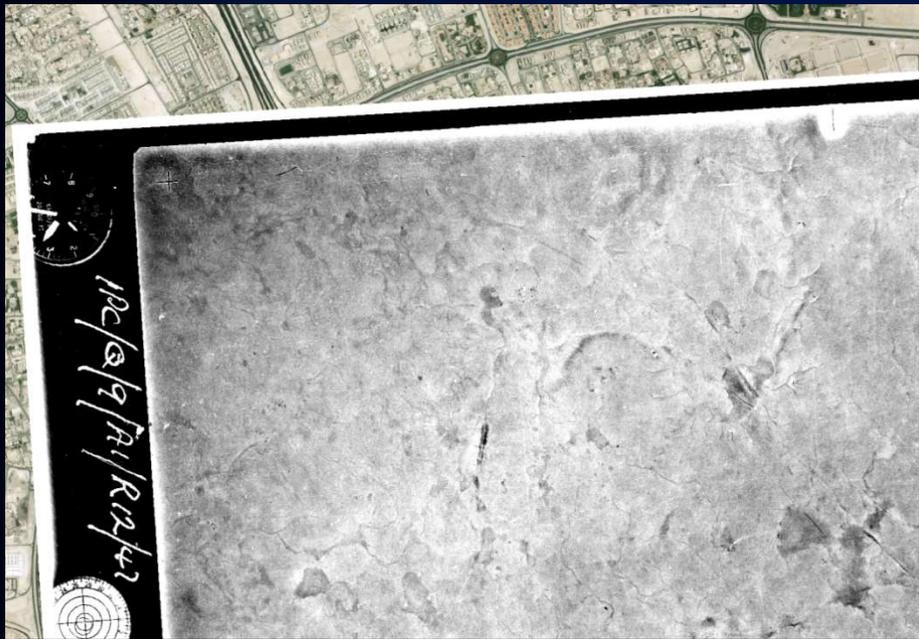
**ABOVE:** The original input data and the importance of date metadata ('47' is 1947). Image shows the 1947 aerial photo and modern satellite imagery before combination through georeferencing.
