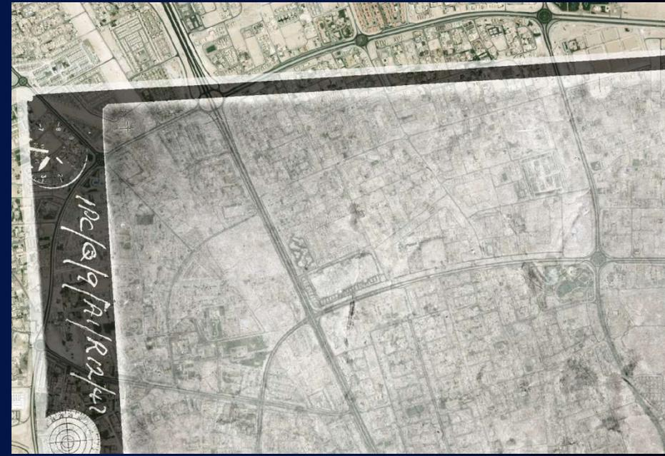
**ABOVE:** Georeferencing 1947 image to identifiable terrain on satellite image. Subsequent building development masks some features. The ability to identify features to reference photos is vital. Need to retain older imagery.
